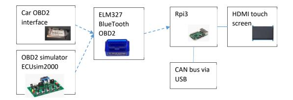
Note: Bluetooth message will be transmitted to CAN bus before arriving at Instrument Cluster application. The purpose is to replace ODB2 completely by CAN interface in Vehicle someday.
